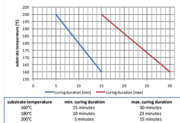
Please observe cure parameters closely since mechanical properties will develop before full cross-linking!
